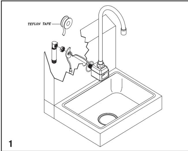
**2 Electronics Module Installation**
