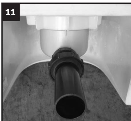
**11** Install the extension tube onto the housing tail pipe and slide the 2" slip joint nut and washer onto the extension tube.
