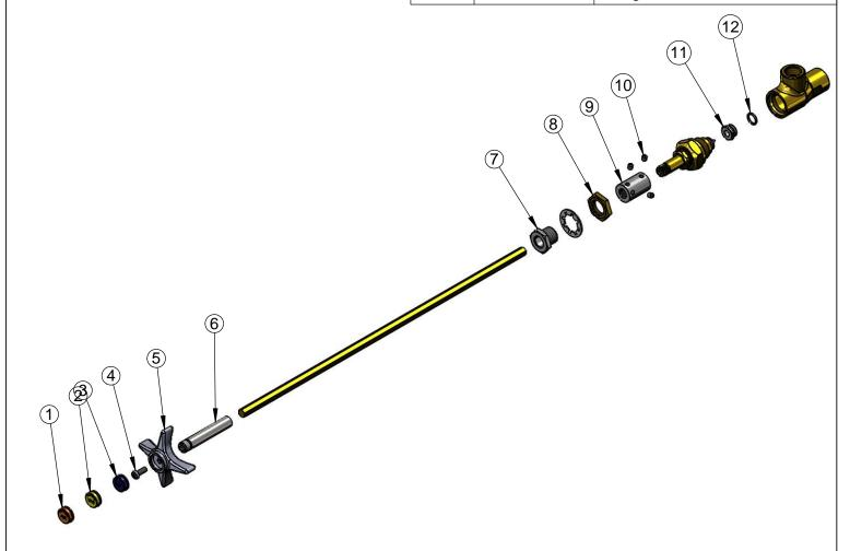
Approved **Product Specifications:** Drawn Checked Remote Control Angled Valve for Gases w/ 18" Centerline to Bushing, 4-Arm Handle, "GAS", "AIR" & "VAC" Snap-In Indexes, "MF" Bushing For Mounting on Metal Surfaces & 3/8" NPT Inlet & Outlet DHL DMH Scale: Date: 09/06/13 NTS
