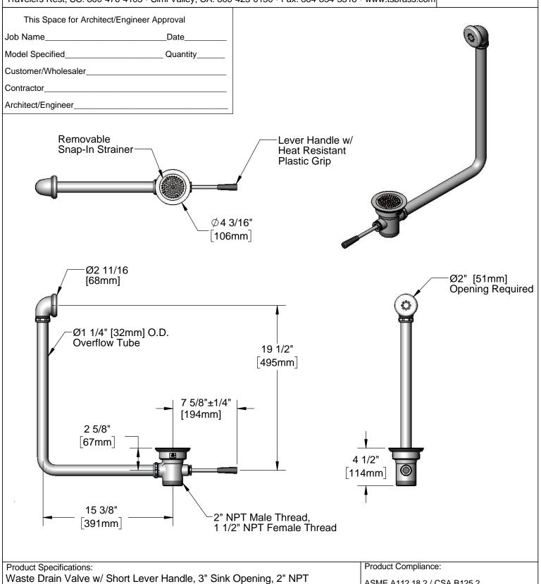
Male Outlet, 1 1/2" NPT Female Outlet & Overflow Tube w/ Head Asm
