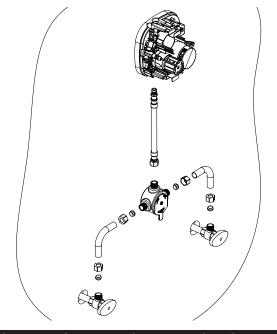
Secure flex hoses to the control module by opening supply hose stainless steel clips.
