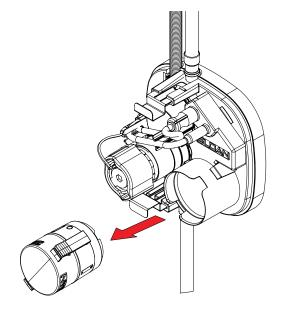
Twist top of battery pack counter-clockwise to open. Remove batteries and replace batteries with four (4) new "AA" batteries. Twist top of battery pack clockwise to close.
