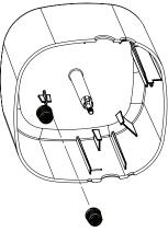
F Snap new filter onto solenoid caddy assembly.
