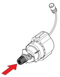
Insert solenoid caddy assembly into control module lining up arrows. Turn solenoid caddy assembly clockwise 45°.
