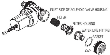
**4. Faucet DOES NOT stop delivering water or continues to drip after user is no longer detected (automatic shut-off fails even when batteries are removed).**
