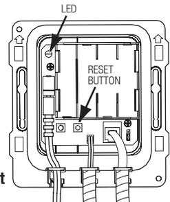
**7. The GREEN LED initially turns on in the control module (below deck) during start up mode, then will not appear again.**
