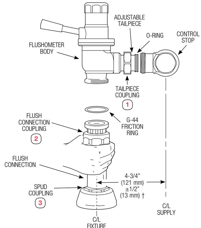
† This measurement can vary +/-1/2” (13 mm) only when an adjustable tailpiece is used.
