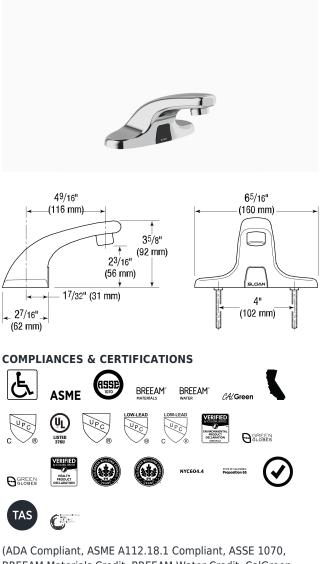
(ADA Compliant, ASME AT12.18.1 Compliant, ASSE 1070, BREEAM Materials Credit, BREEAM Water Credit, CalGreen Compliant, CEC Compliant, cUPC Certified, UL Certified, UPC Certified, UPC Low Lead Compliant, cUPC Low Lead Compliant, EPD, Green Globes Materials & Resources Credit, Green Globes Water Credit, HPD, LEED Materials & Resources EPD Credit, LEED Materials & Resources HPD Credit, NYC604.4, Proposition 65, Satisfies LEED Credits, TAS, WELL Building Standard)
