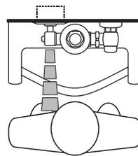
3. When the user steps away from the OPTIMA® Sensor, the circuit immediately initiates an electrical "one-time" signal that operates the Solenoid. This initiates the flushing cycle to flush the fixture. The Circuit then automatically resets and is ready for the next user.
