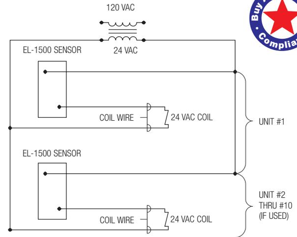
One Transformer serves up to ten (10) OPTIMA® Closet/Urinal Flushometers. Specify number of transformers required accordingly.
