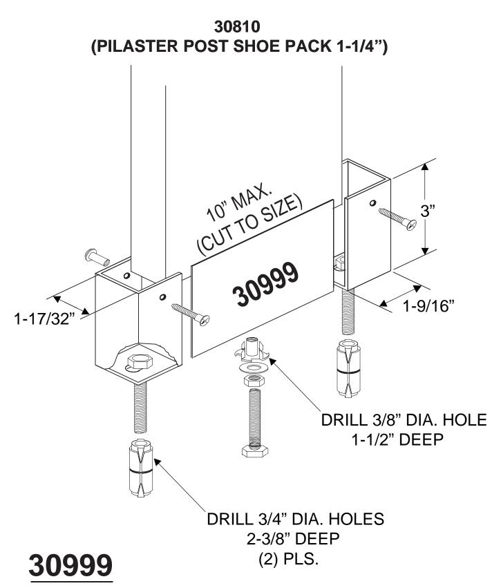
Stainless steel spacer plates must be ordered seperately and measure 3" X 10".
