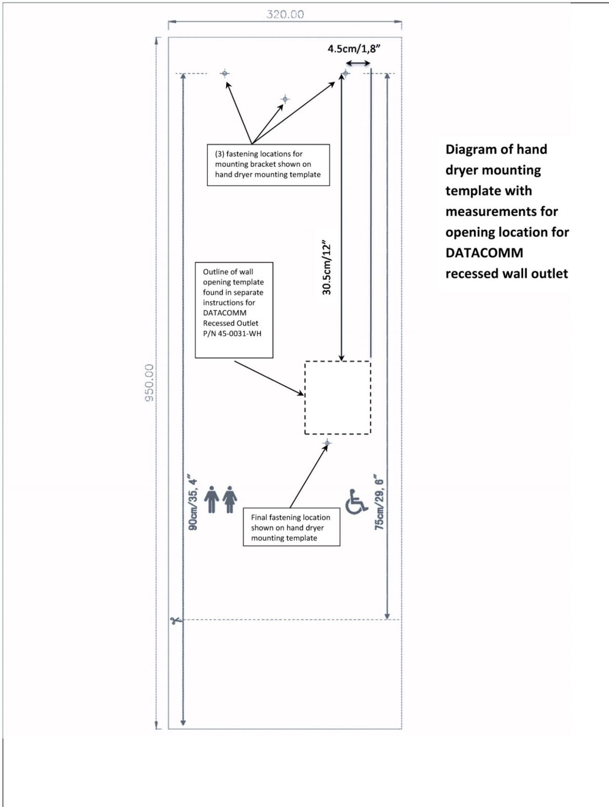
Fig. 1: Mounting Location for Recessed Duplex Receptacle
