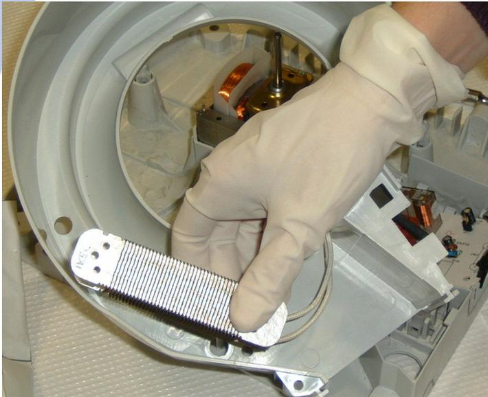
← Step 7: Remove the heating element from its housing.
