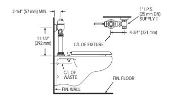
NAVAL 120, 121 & 122 — Water Saver, 3.5 gpf (13.2 Lpf) NAVAL 120-1.6, 121-1.6 & 122-1.6 — Low Consumption, 1.6 gpf (6.0 Lpf)
