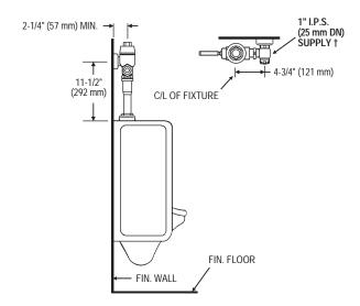
† 1" CONTROL STOP IS AVAILABLE WITH WHITWORTH THREAD
