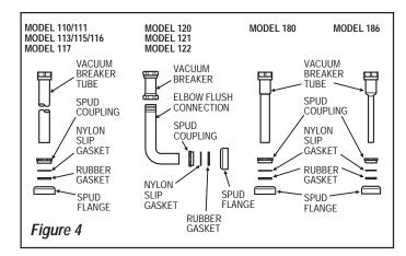
tube to the bottom of the valve using the slip gasket supplied.
