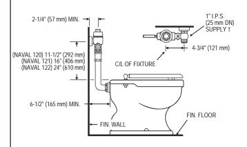
† 1" CONTROL STOP IS AVAILABLE WITH WHITWORTH THREAD
