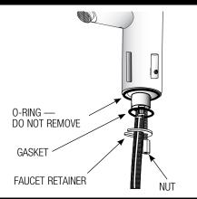
Install Faucet with 0-ring into the center hole in deck or lavatory — 1-3/16" (30 mm) min. hole required.
