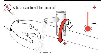
B Optional — To fix temperature, set lever to the desired position, then remove lever and plug hole with Cap.
