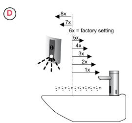
DISCLAIMER: Updated electronics have visible red and green LED. Original electronics have only red LED and range setting is reversed (1=longest, 8=shortest)
