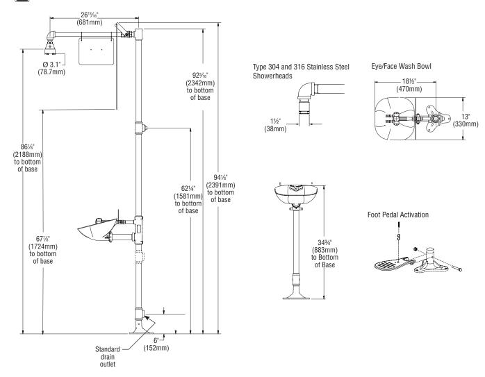
All dimensions assume standard thread engagement. Variations in manufacturing allow for +/- 1/8"(3mm) per threaded joint. To find the tolerance of a dimension, add the number of thread joints across the length of the dimension and multiply it by 1/8" (3mm).
