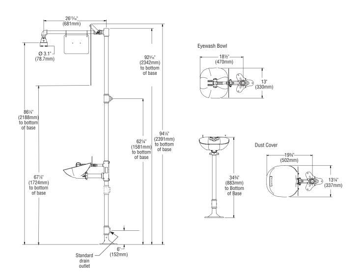
All dimensions assume standard thread engagement. Variations in manufacturing allow for  $+/- \frac{1}{6}$ " (3mm) per threaded joint. To find the tolerance of a dimension, add the number of thread joints across the length of the dimension and multiply it by  $\frac{1}{6}$ " (3mm).
