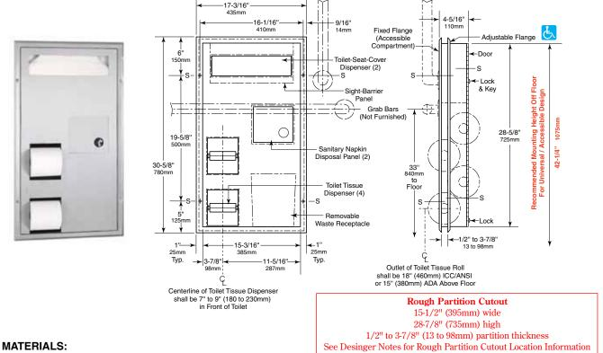
Cabinet — 18-8 S, type-304, heavy-gauge stainless steel. All-welded construction. Exposed surfaces have satin finish. Equipped with a plastic sight-barrier panel for the toilet-seat-cover dispenser.
