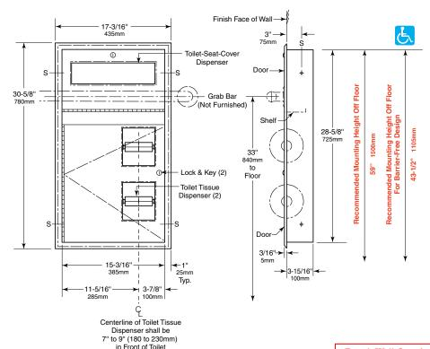
Rough Wall Opening 16" (405mm) wide 29-1/4" (745mm) high 4" (102mm) minimum recessed depth
