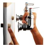
Step 1: Apply plumber's putty to backside of body and insert into mounting hole. Line up water supply lines and couplings, attach and tighten with wrench.
