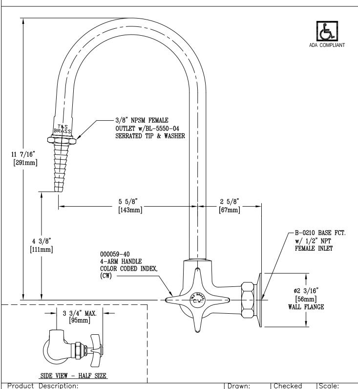
WALL MOUNTED SINGLE SUPPLY FAUCET w/ RIGID GOOSENECK, 4-ARM HANDLE, SERRATED TIP & 1/2" NPT FEMALE INLET
