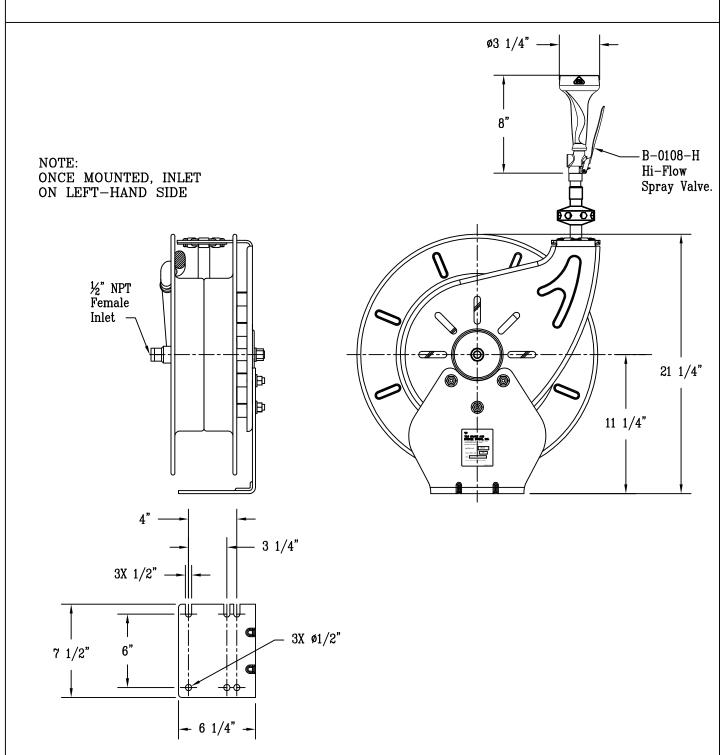
Hose Reel: Open, Epoxy Powder Coated Steel, 50 FT of 1/2" Dia. Blue Hose and
