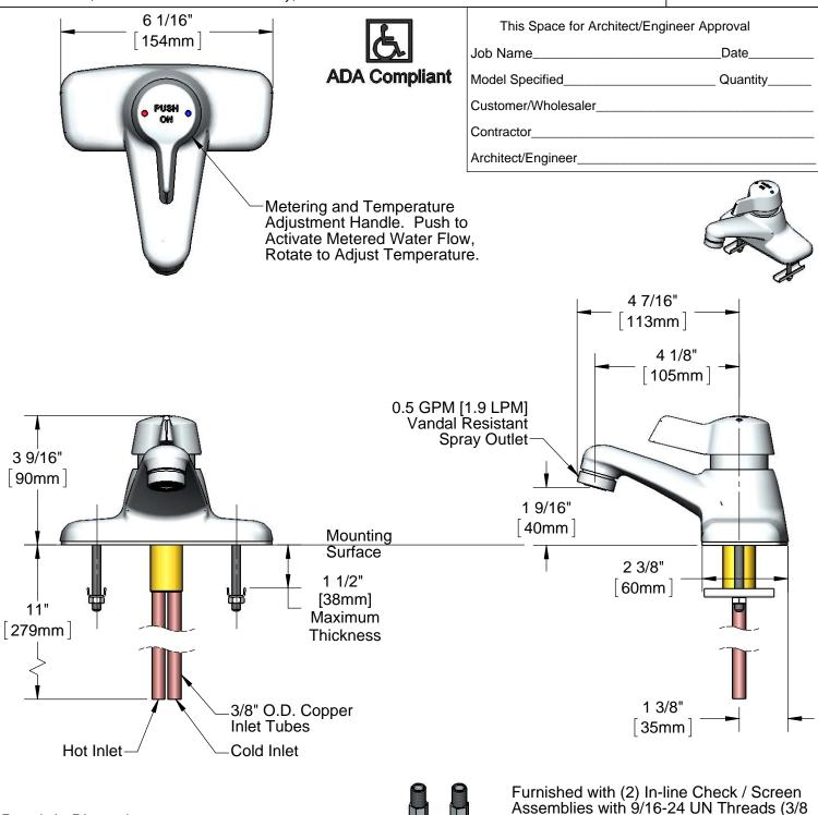
Rough-In Dimensions: (3) Holes on 2" Centers, Ø1" Min. for Center Hole
