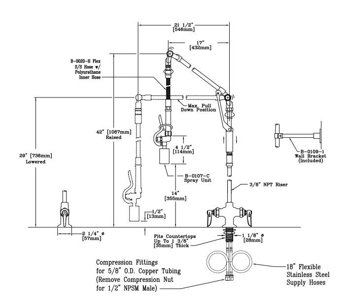
NOTE: For Backsplash Mounting, Riser Must Be Shortened To Maintain 14" [356mm] Clearance Between Spray Head And Fixture Flood Rim Level
