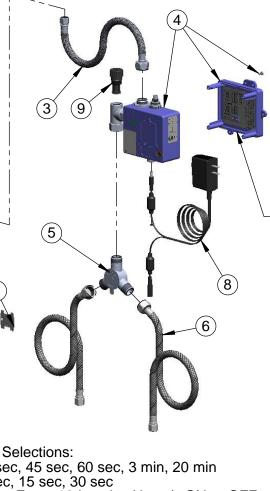
A Maximum of (8) ChekPoint Faucets can be Hardwire Connected and Powered by EC-HARDWIRE ChekPoint Hardwire AC Transformer. (Sold Separately)
