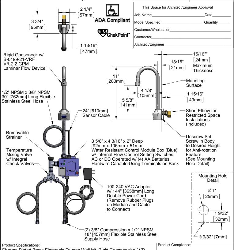
Chrome Plated Brass Electronic Faucet: Wall Mt. Rigid Gooseneck w/ VR 2.2 GPM Laminar Flow Device, AC/DC Control Module with Internal Flow Control Setting Switches, Temperature Control Mixing Valve w/ Integral Check Valves, 18" Flexible Stainless Steel Supply Hoses
