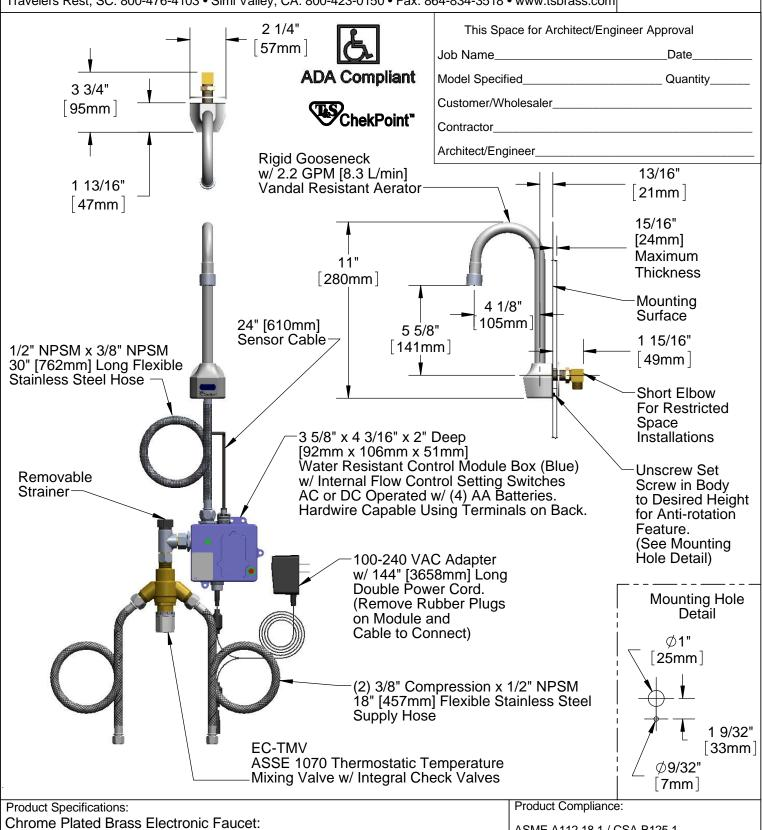
ASSE 1070 Drawn: GEF Checked: DMH Approved: Date: 05/07/14 Scale: 1:6 Sheet: 1 of 2
