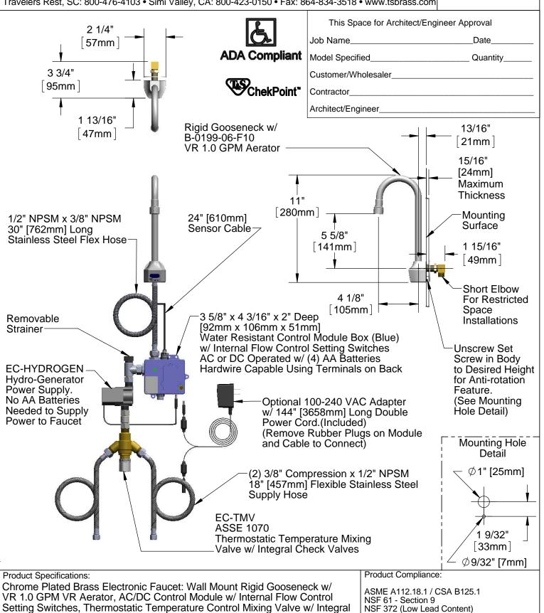
Setting Switches, Thermostatic Temperature Control Mixing Valve w/ Integral Check Valves, Hydro-Generator, 18" Lg Hot & Cold Supply Stop Flexible
