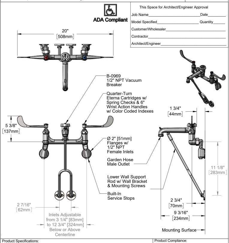
Adjustable Wall Mount Service Sink Faucet, Quarter-Turn Eterna Cartridges w/ Spring Checks, 6" Wrist Action Handles, Lower Support Rod, 1/2" NPT Adjustable Inlets w/ Supply Stops, Male Garden Hose Outlet, Polished Chrome Finish & 1/2" NPT Vacuum Breaker
