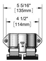
3 9/16" [90mm] Closed 2 7/16" 25mm 61mm 2 5/8" 2 1/4" 1 15/16" [67mm] [57mm] [49mm] 4 1/4" [108mm] 1/2" NPT Closed Female Inlet 1/2" NPT Female 4 5/16" Outlet [109mm] Knee Pedals Hang Outside of Cabinetry for Knee Access
