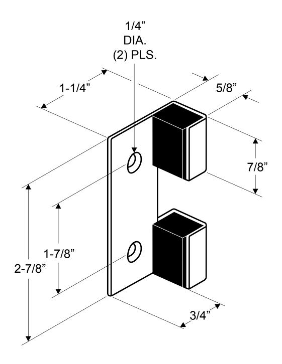
NOTE: FLAT-BACKED FOR WALL MOUNTING. 14 GAUGE (.075" THICK STAINLESS)
