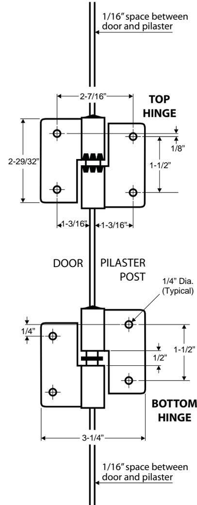
1. Locate and set hinge leaves to pilaster post as per drawing.
