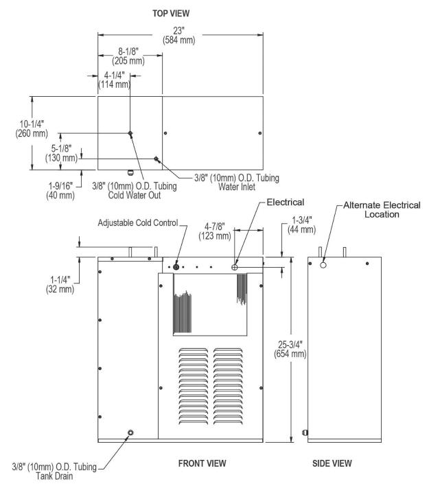
**NOTE:** It is important to insure proper ventilation. Allow a minimum clearance of 12" (305mm) in front and 3" (76mm) in the rear of unit.
