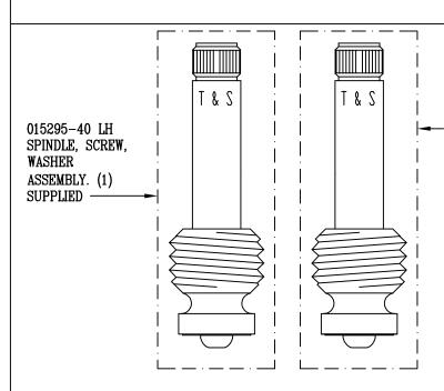
·015294-40 RH SPINDLE, SCREW, WASHER ASSEMBLY. (1) SUPPLIED
