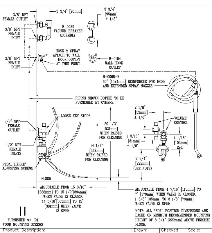
BED PAN WASHER WITH SINGLE PEDAL FOOT VALVE, INTEGRAL LOOSE KEY STOPS, VACUUM BREAKER, & HEAVY DUTY RUBBER HOSE W/ EXTENDED SPRAY OUTLET
