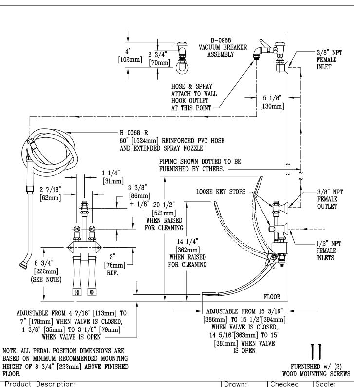
BED PAN WASHER WITH FOOT VALVE CONTROL,
