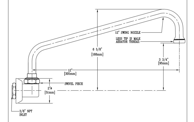
WALL MOUNTED DUMMY GOOSENECK WITH 62X 12" SWING NOZZLE
