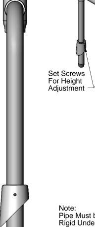
Note: Pipe Must be Held Rigid Under Sink by Connection Fittings, Brace, Etc.
