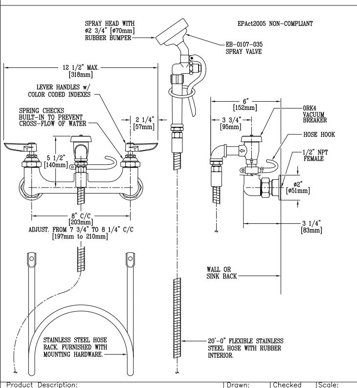
POT & KETTLE FILLER: EB-0107-035 SPRAY VALVE w/ FLEX HOSE ASM, B-131 FAUCET BASE, LEVER HANDLES & VACUUM BREAKER
