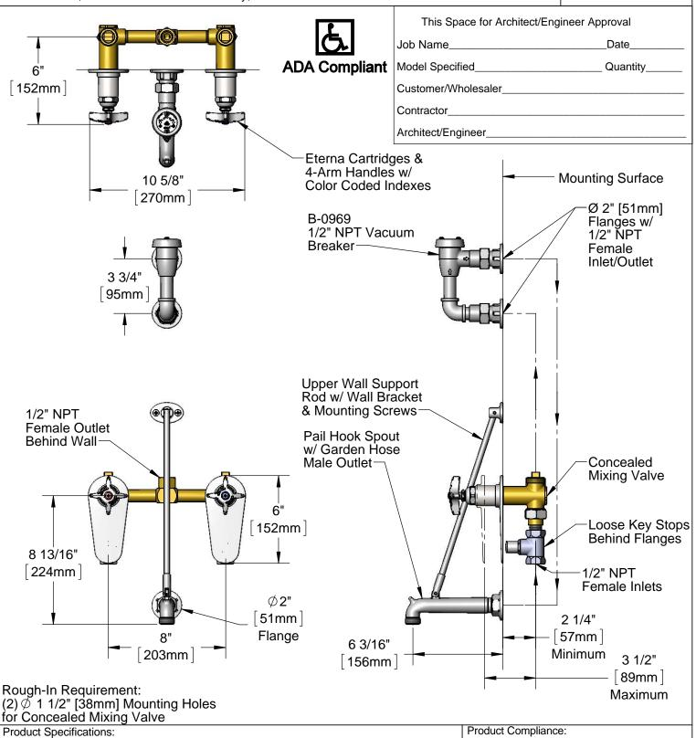
8" Wall Mount Concealed Mixing Valve, Eterna Cartridges, 4-Arm Handles, Loose Key Stops, Elevated Vacuum Breaker, Spout w/ Garden Hose Male Outlet & Upper Support Rod & 1/2" Female Inlets/Outlets
